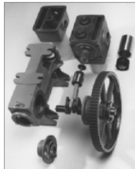
Disassembled pump showing the major parts
